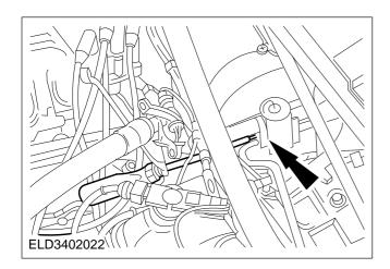
5. Disconnect the line from the expansion valve.
