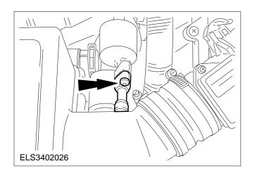
4. Detach the seal retaining plate.
