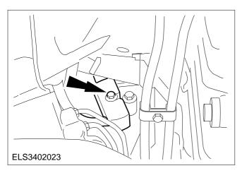
4. Disconnect the line from the compressor. Remove the O-ring.
