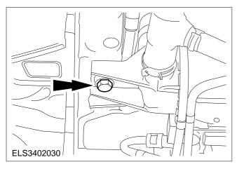
5. Unscrew the refrigerant line at the line connector.
