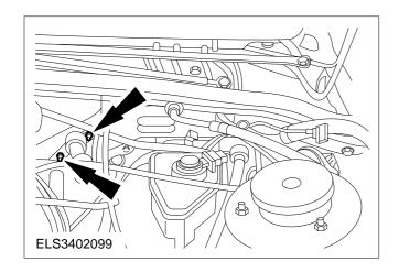
10. Detach the seal retaining plate.
