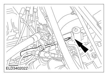
11. Disconnect the line at the expansion valve.
