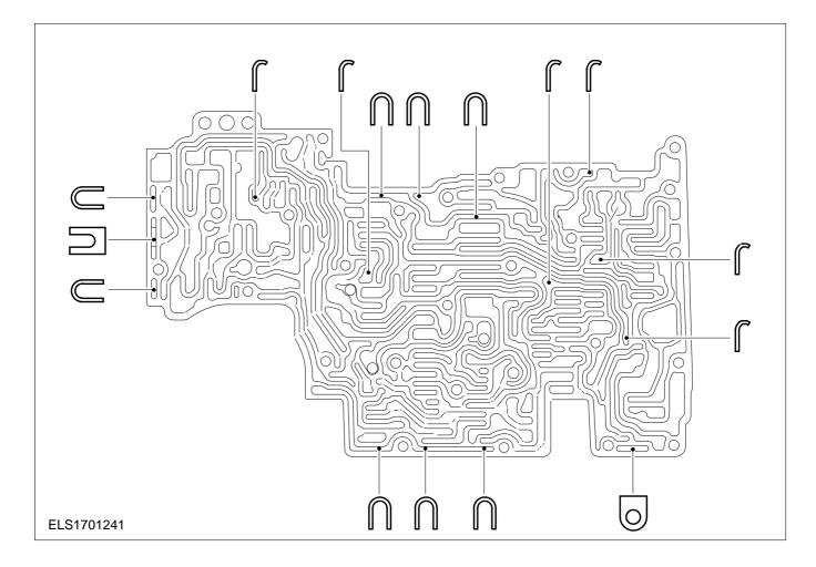
NOTE: Installation position of the retaining pins.
