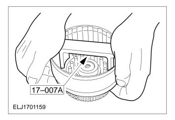
Assemble the forward clutch
