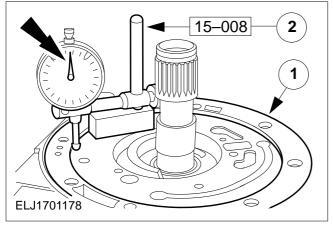
Measure the end float of the O/D gear train.
