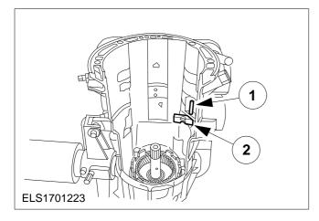
37. Remove the input bell housing.
