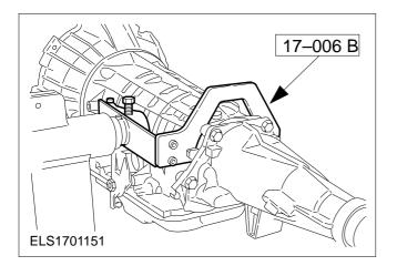
2. Withdraw the input shaft.
