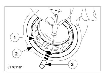
Install the one-way clutch of the rear gear train
