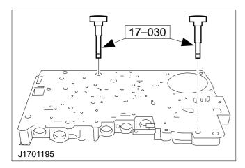
Assemble the valve body assembly
