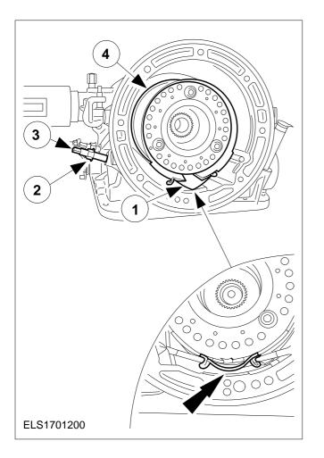
**NOTE:** Mark the O/D brake band to prevent it being mistaken for the centre brake band.
