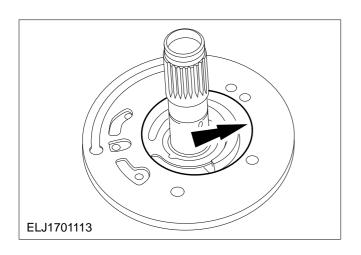
**NOTE:** The transmission fluid pump can only be renewed as a complete unit.
