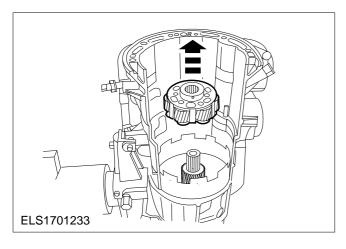
33. Remove the reverse and direct drive clutch.
