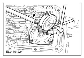
Check the length of the rear servo piston rod
