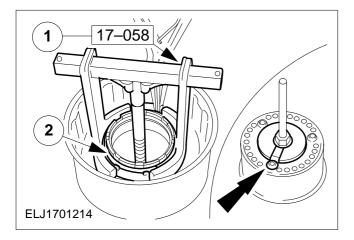
**NOTE:** Align the recess on the special tool with the ball valve.
