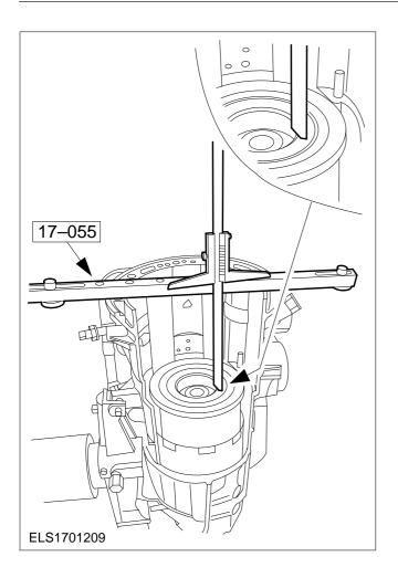
Measure the end float of the rear gear train
