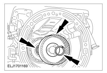
Remove the seal of the transmission extension housing
