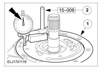
Check the end float of the O/D gear train
