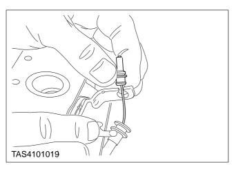
7. Unclip and remove the hood release cable.
