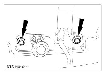
5. Remove the catch retaining bolts.
