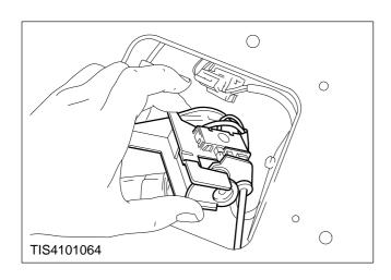
4. Ease the actuator mechanism out from the compartment lid to access the barrel spacer tube.
