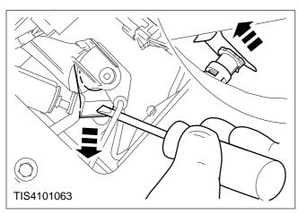
3. Remove the barrel retaining clip.
