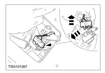
8. Disconnect the barrel set/reset switch and remove the actuator mechanism.
