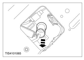
5. Remove the spacer tube.
