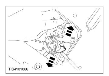
7. Disconnect the lock actuating rod.
