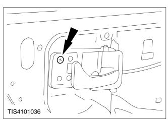
4. Remove the remote control handle retaining screw.
