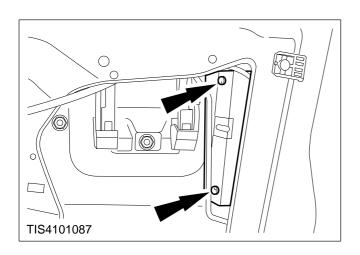
5. Remove the barrel lock shield (two screws).
