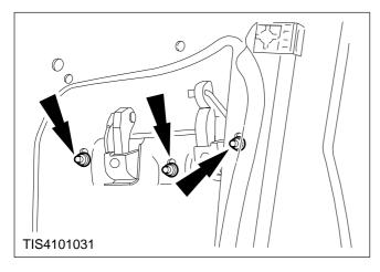
7. Remove the three handle retaining nuts.
