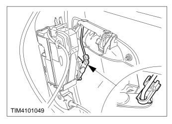
6. Disconnect the door lock actuating rod.
