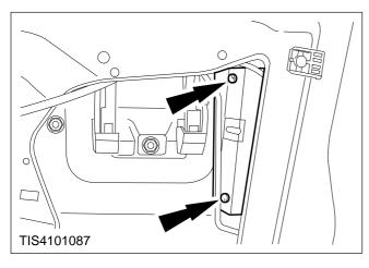
7. Remove the barrel lock shield (two screws).
