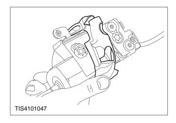
Motor – Lock – Front Door – Remove (33 779 0)
