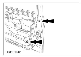
10. Displace the door window guide channel for access.
