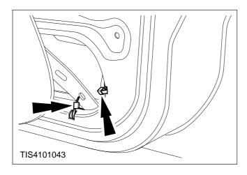
11. Unclip the two lock harness cable ties to allow cable movement.
