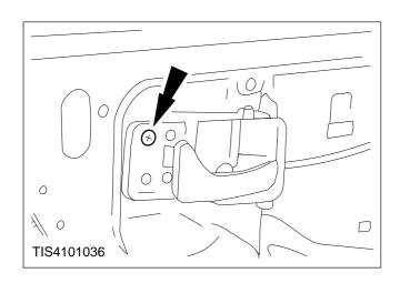
5. Detach the remote control handle (one retaining screw).
