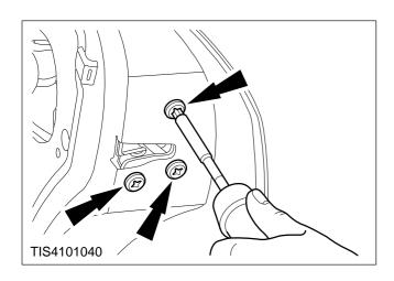
9. Remove the three lock retaining screws.
