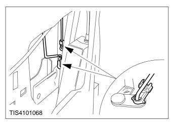
8. Disconnect the door handle and barrel actuating rods.
