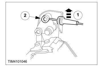
9. Disconnect the door handle actuating rod.
