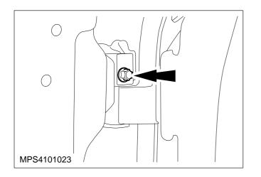
4. Remove the two hinge pin torx bolts.
