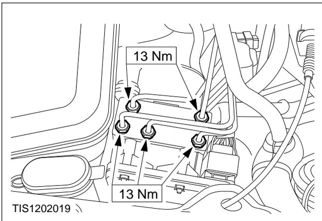
**6. Bleed the braking system as described in Operation No. 12 141 0.**
