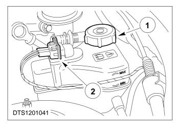
2. Remove the filler cap and disconnect the warning indicator multiplug.
