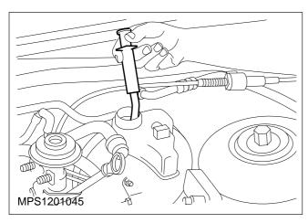
3. Using a suitable syringe remove as much fluid as possible from the reservoir.
