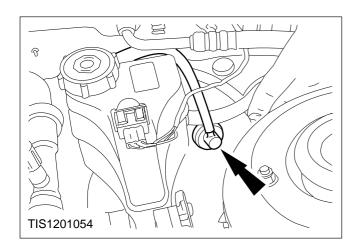
4. Carefully detach the vacuum hose from the servo housing.
