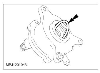
5. Remove the pump to alternator 'O' ring.
