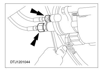
**NOTE:** Blank off the pipes to prevent any dirt ingress.
