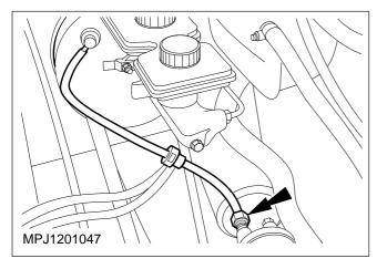
2. Disconnect the vacuum hose from the vacuum pump.
