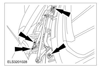
5. Detach the wiper motor complete with the linkage.
