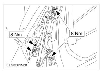
12. Fit the wiper motor complete with the linkage.
