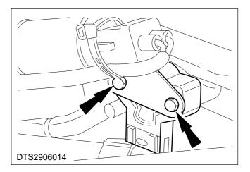
3. Remove the throttle position sensor (two bolts).
