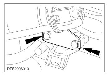
2. Unlock the throttle position sensor retaining bolt locking tags.
