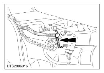
4. Remove the vehicle speed sensor wiring loom cable tie.
