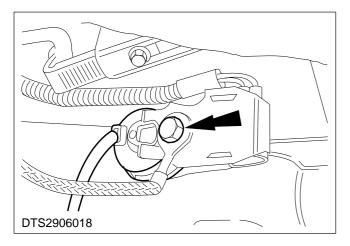
5. Disconnect the vehicle speed sensor multiplug.
