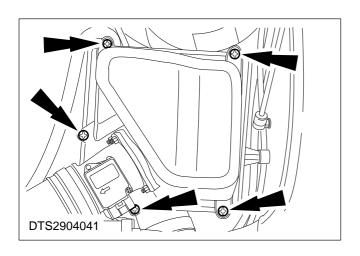
4. Remove the air cleaner assembly cover retaining screws.
