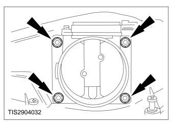
6. Remove the sensor retaining nuts.
