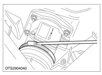
3. Disconnect the air induction pipe from the MAF sensor.
