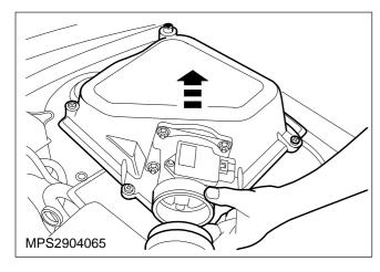
5. Lift the cover off complete with the MAF sensor.
