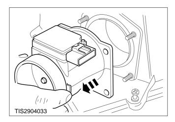
7. Separate the sensor from the air cleaner assembly cover.
