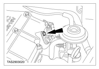
2. Unscrew the CMP sensor retaining bolt.
