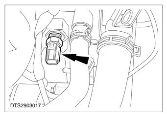
7. Unscrew and remove the ECT sensor (2,3 DOHC shown).
