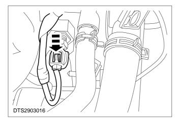
6. Disconnect the ECT sensor multiplug (2,3 DOHC shown).
