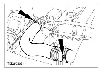
2. Slacken the hose clips and remove the intake hose.
