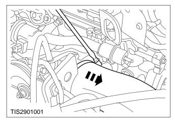
3. Slacken the clip and disconnect the intake hose.
