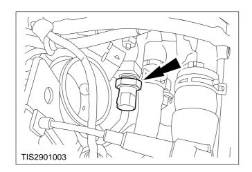
5. Unscrew and remove the ECT sensor.
