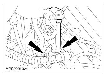
3. Unscrew the IAC valve retaining bolts.
