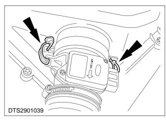
3. Release the MAF sensor retaining clips.
