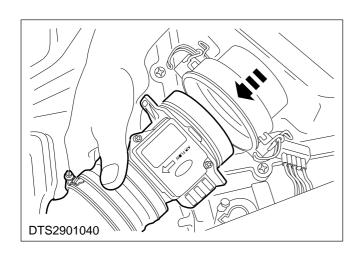
4. Disconnect the MAF sensor from the air cleaner housing.
