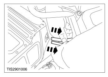
2. Disconnect the pressure transducer EGR system hoses.
