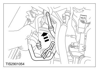
6. Remove and discard the exhaust manifold to EGR valve pipe.
