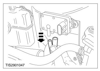
3. Disconnect the pressure transducer EGR system hoses.
