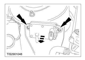
4. Unscrew the pressure transducer EGR system retaining screws.
