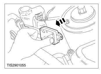
5. Remove the pressure transducer EGR system.
