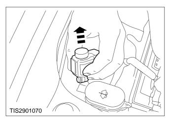
6. Unclip and remove the VIS vacuum regulator.
