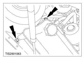
2. Unscrew the degas tank retaining bolts.
