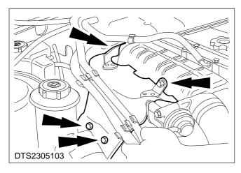
**WARNING:** The exhaust manifold and heatshield may be hot.
