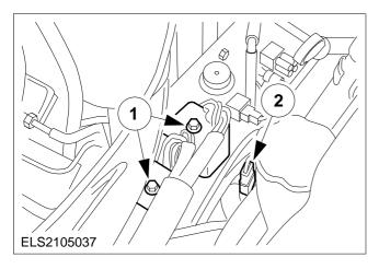
83. Attach the upper oil pipe to the oil cooler.
