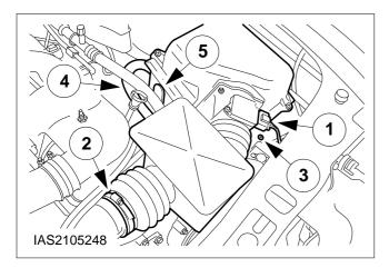
5. Remove the cover from the intake system.
