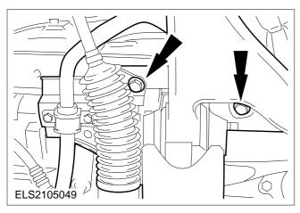
30. Detach the engine mounting (left-hand side shown).
