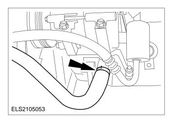
**39.** Detach the coolant hose at the bottom.
