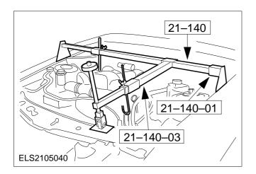
53. Unhook the engine support bracket from the engine lifting eyes and carefully raise the vehicle.
