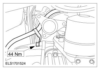
56. Attach the wiring bracket to the transmission.
