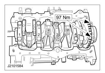
**NOTE:** Fit the bolts with the threaded pins in bearings 3 and 5.
