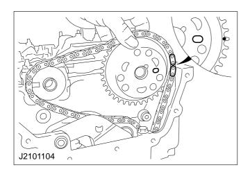
81. Tighten the timing chain guide rail bolts.
