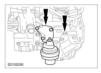
104. Install the brackets for the air conditioning compressor and the exhaust.
