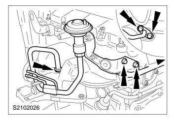
2. Detach the engine mounting bracket with the engine mounting.
