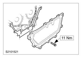
**NOTE:** The upper edge of the cover must be a maximum of 0,13 mm below the mating face of the cylinder head cover.
