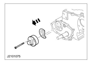
NOTE: Release the three auxiliary bolts first.
