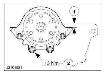
Install the rear oil seal housing
