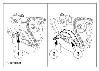
23. Remove the camshaft sprockets.
