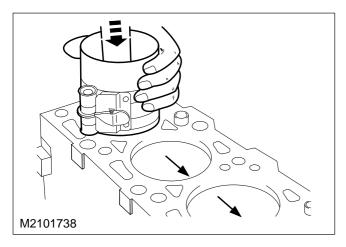
**CAUTION:** The maximum width of the piston rings corresponds to the diameter of the cylinder bore + 1,7 mm.
