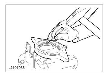
54. Remove the oil seal from the rear oil seal housing.
