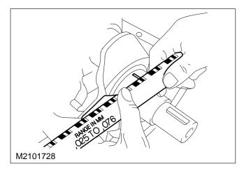
**CAUTION:** The crankshaft must not be turned during the measuring operation.
