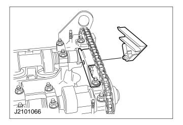
**NOTE:** The chain guide must be renewed during installation.
