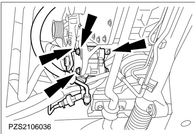
**27. Detach the power steering pump and tie it up.**
