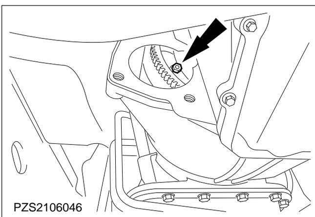
**NOTE:** Ensure the torque converter is correctly fitted in the engine drive plate.
