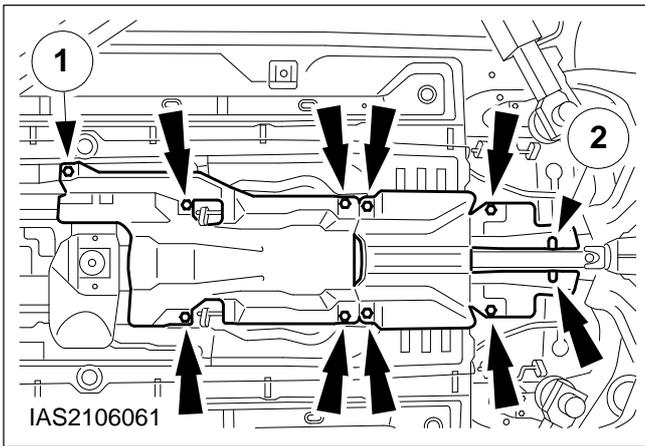
**34. Detach the exhaust system heat shields.**
