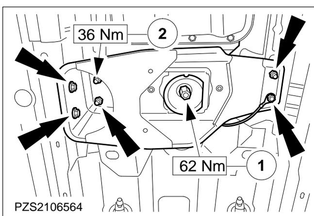
**74. Raise the automatic transmission using the transmission jack.**
