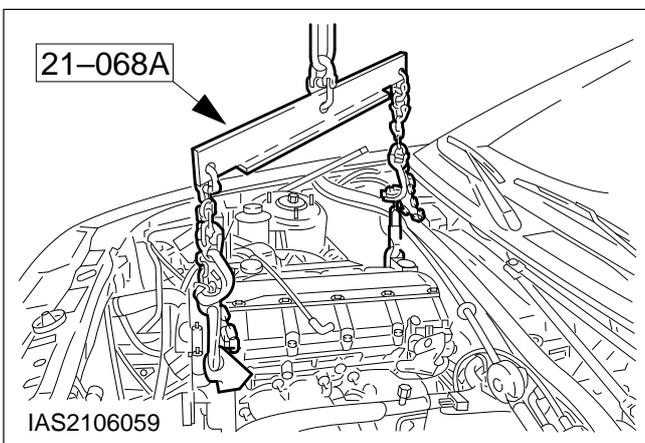
50. Attach the engine lifting bracket.
