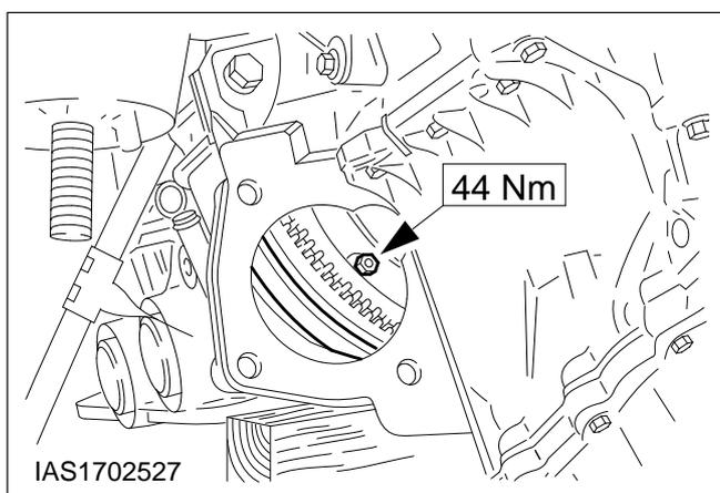
**66. Secure the torque converter.**
