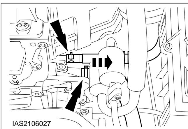
**14. Detach the coolant hoses from the coolant pump.**
