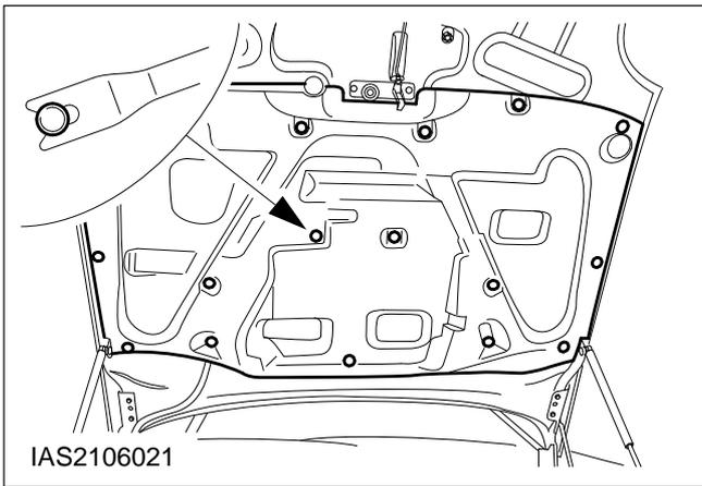
**6. Remove the hood insulation panel (17 expanding pins).**
