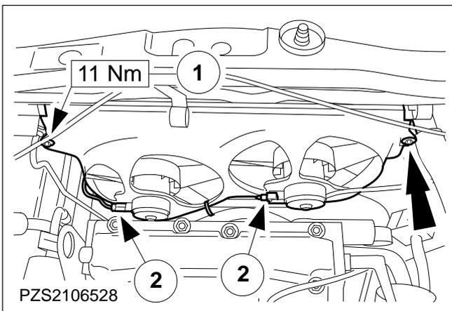
**110. Install the fan motors with the air baffle.**
