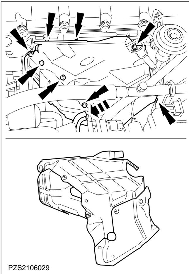
**16. Remove the three-part exhaust manifold heatshield.**
