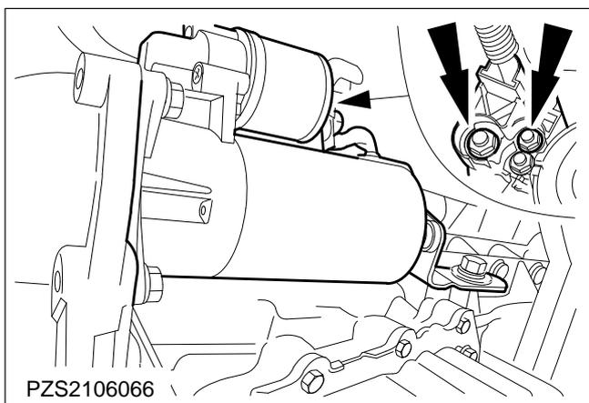
**87. Connect the starter motor lead.**
