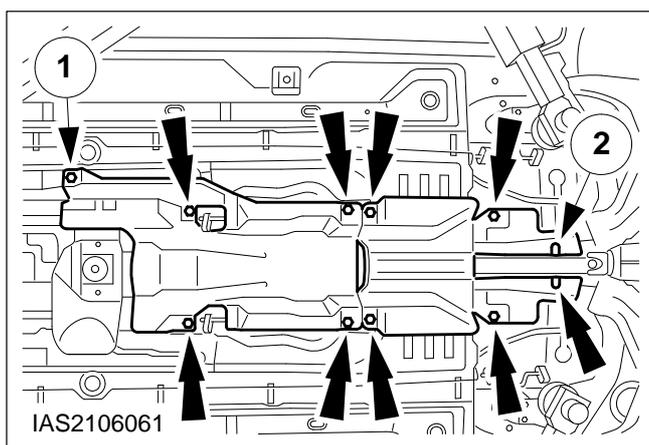
**80. Fit the exhaust system heat shields.**
