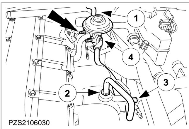
**18. Detach the exhaust gas recirculation valve (EGR valve) and the EGR pipe.**
