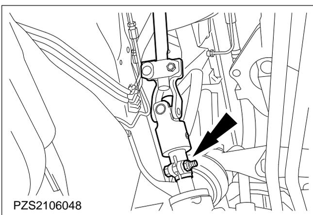
**45. Detach the steering intermediate shaft.**
