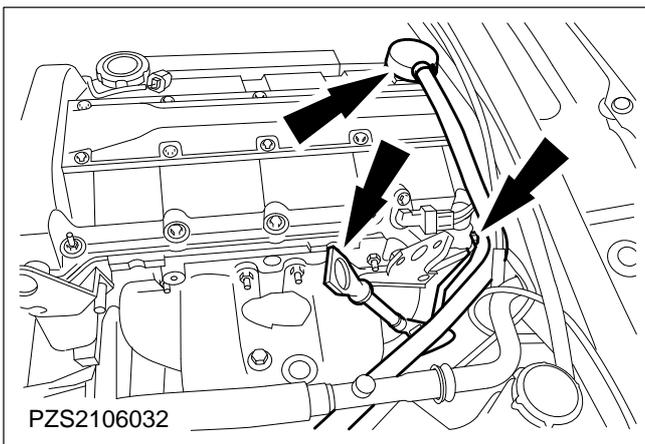
**20. Remove the valve with the crankcase breather hose and unclip it.**
