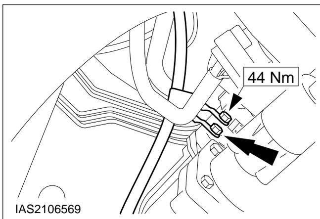
**86. Fit the oil dipstick tube and the earth lead.**
