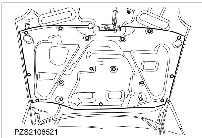
**119. Fit the hood insulation panel (17 expanding pins).**
