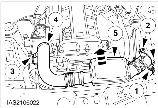
**8. Remove the intake pipe.**
