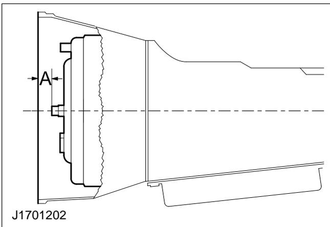
**62. Check the fitted measurement of the torque converter:**
