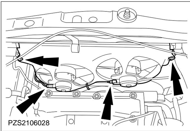
**15. Remove the fan motors and air baffle complete.**
