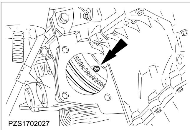
**54. Detach the torque converter from the engine drive plate (four nuts).**
