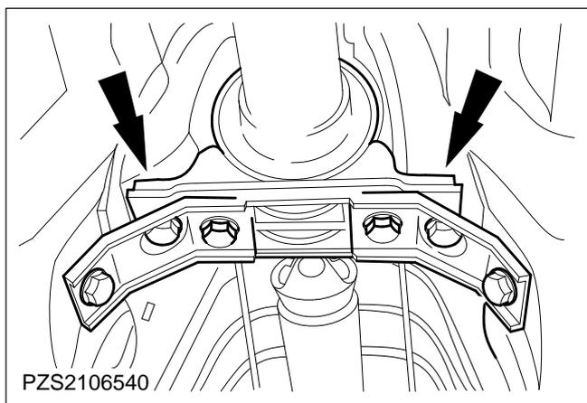
**76. Push the driveshaft into the automatic transmission.**
