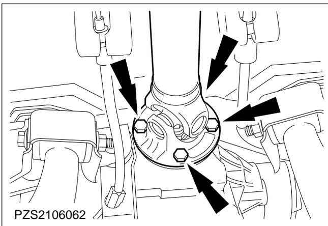
**35. Detach the driveshaft from the rear axle.**
