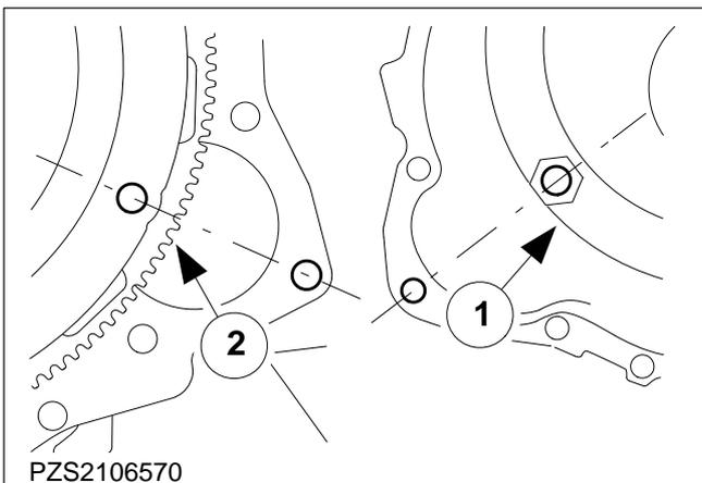
**61. Move the torque converter into the installation position on the automatic transmission and the drive plate into the installation position on the engine.**
