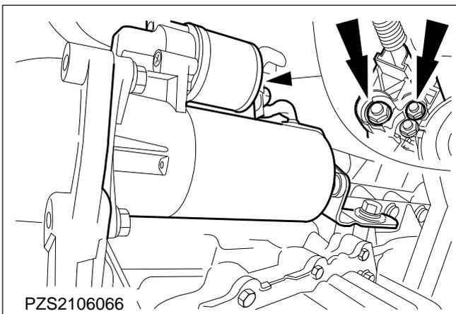
**40. Disconnect the starter motor lead.**
