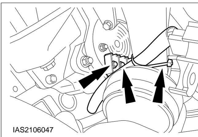
**44. Disconnect the alternator lead.**
