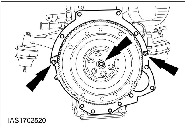
**58. If necessary move the locating sleeves from the automatic transmission flange to the engine flange.**
