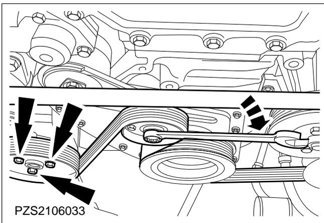
**22. Loosen the power steering pump pulley.**
