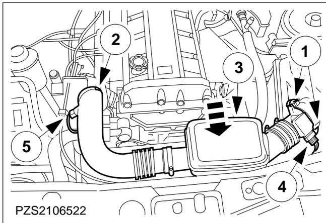
**117. Install the air intake pipe.**
