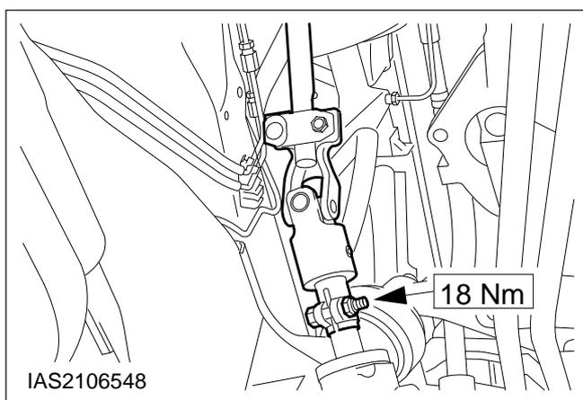
**82. Connect the steering intermediate shaft.**
