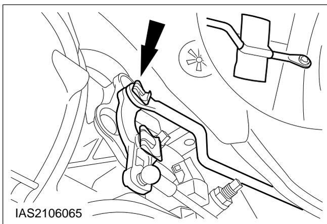
**73. Attach the shift rod to the cranked lever.**
