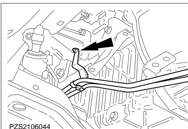
**41. Detach the bracket for the oil pipes.**
