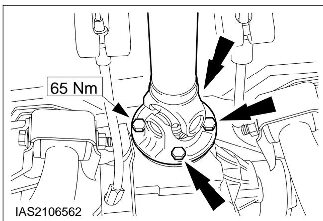
**78. Attach the driveshaft to the rear axle.**
