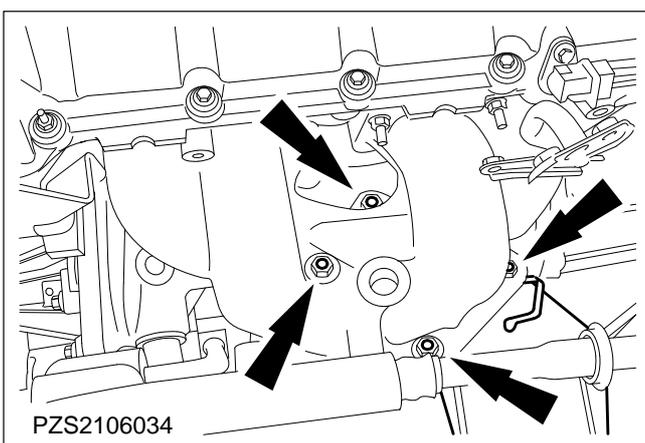
**24. Detach the catalytic converter from the exhaust manifold.**
