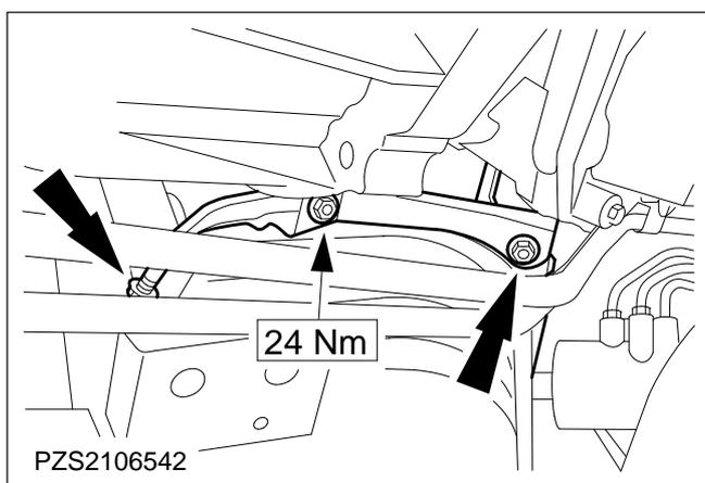
**95. Fit the front catalytic converter bracket.**
