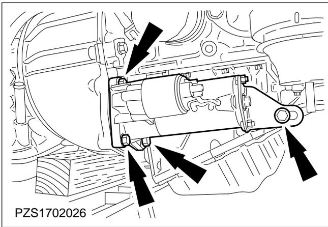
**53. Remove the starter motor and bracket.**
