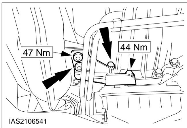
**96. Attach the bracket to the automatic transmission and the catalytic converter.**
