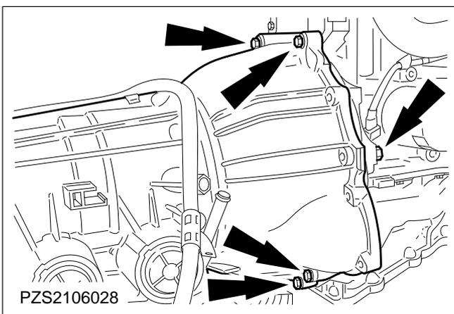
**55. Disconnect the automatic transmission from the engine.**
