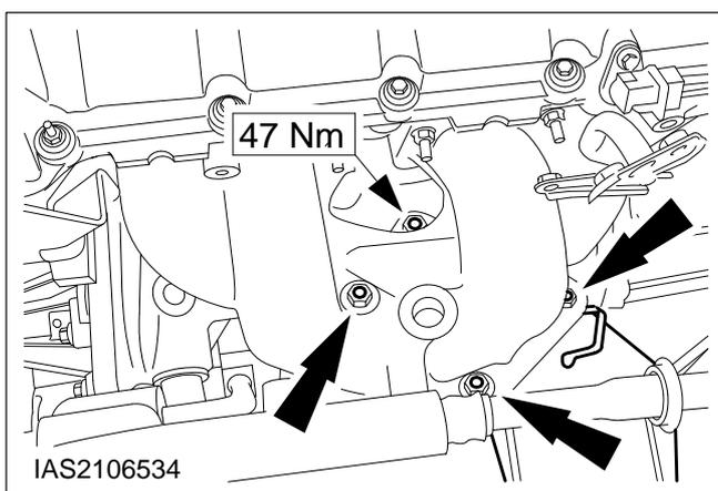
**88. Move the catalytic converter with the front exhaust pipe and with a new gasket into the installation position.**
