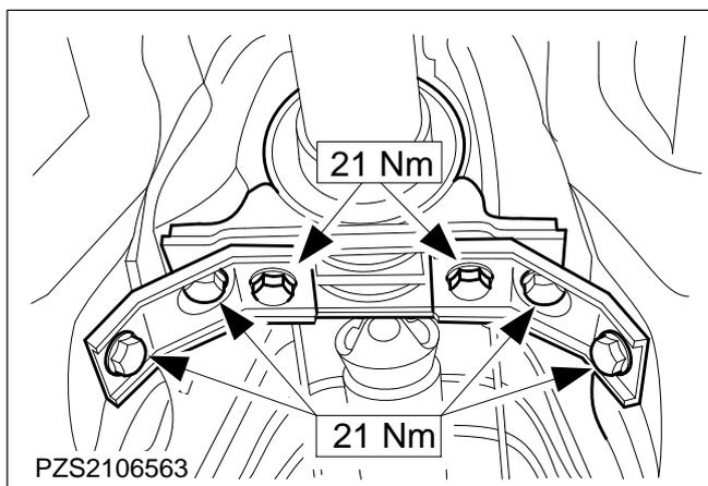
**79. Align the centre bearing so that it is free of strain and tighten it.**
