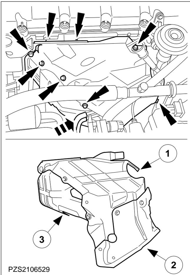
**108. Fit the three-part exhaust manifold heatshield.**
