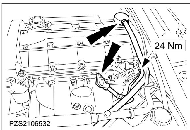
**104. Connect the valve with the crankcase breather hose and clip it into place.**
