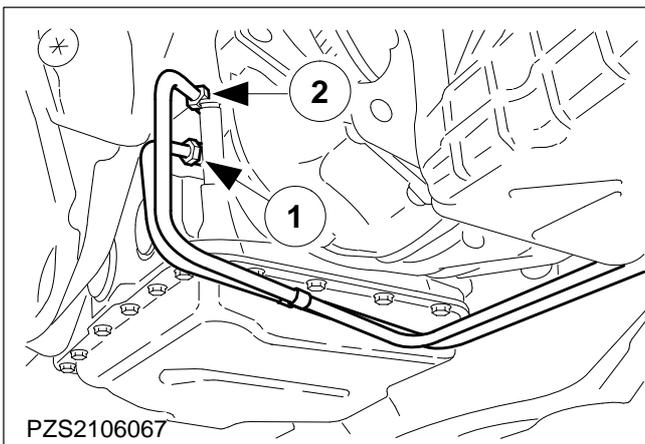
**43. Detach the oil pipes from the automatic transmission.**
