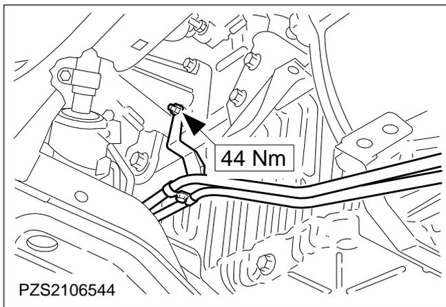
**85. Attach the bracket for the oil pipes.**
