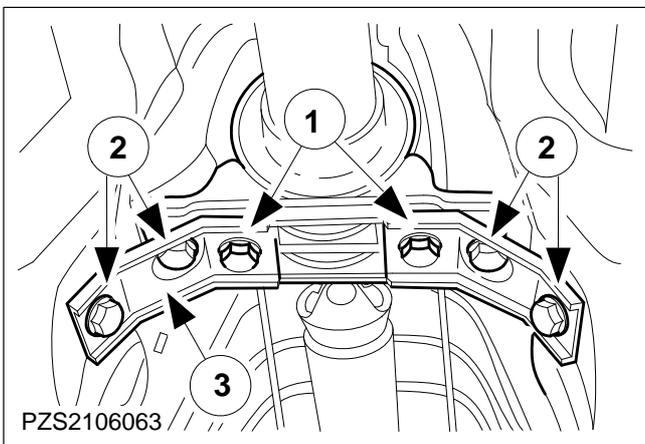
**36. Detach the driveshaft centre bearing.**
