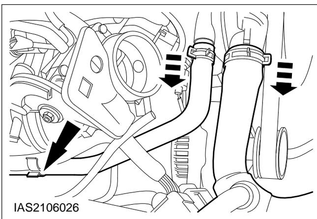
**13. Detach the coolant hoses from the thermostat housing.**
