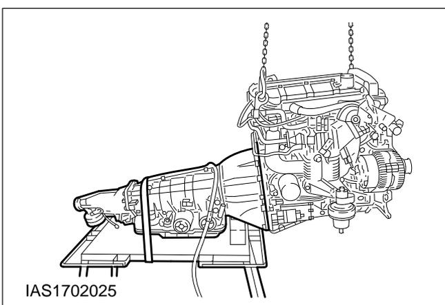
Engine from/to Automatic Transmission –
