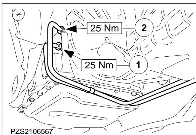
**84. Attach the oil pipes to the automatic transmission.**
