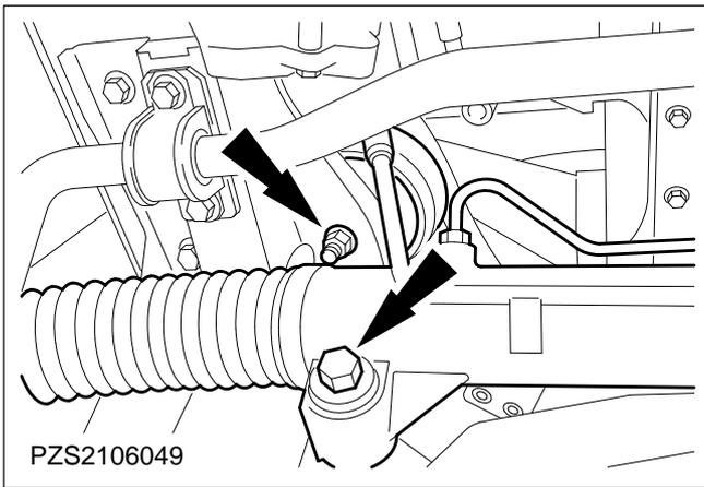
46. Detach the steering gear (one bolt on either side) and lower it.
