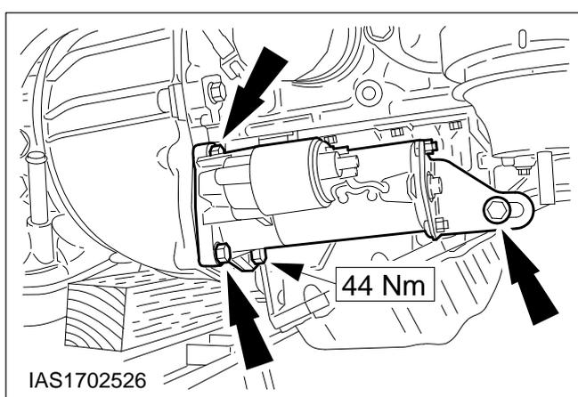
**67. Fit the starter motor and bracket.**
