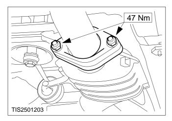
CAUTION: Never use jointing compound forward of the catalyst when installing exhaust components.
