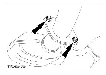
3. Disconnect the catalyst from the front exhaust system flange (two nuts).
