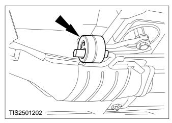
**NOTE:** If the catalyst is to be refitted care must be taken not to damage the assembly, excessive force may damage the ceramic substrates.
