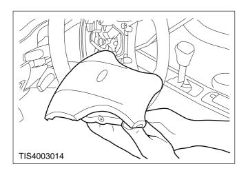
WARNING: Always carry the module with the cover side away from the body and stand it with the cover uppermost. Do not attempt to repair/open or apply electrical power to the module. Never use modules that are visibly damaged. Do not expose the module to heat sources in excess of 100°C.
