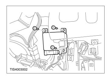
4. Remove the three retaining bolts.
