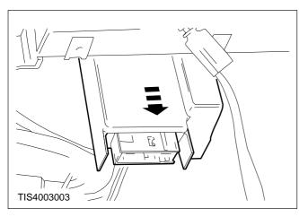
5. Remove the air bag control module from the vehicle.
