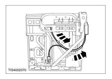
CAUTION: Make sure the routing of the two Bowden cables is noted before removing the assembly.
