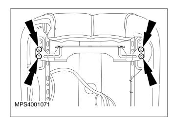
4. Remove the seat base front support bar.
