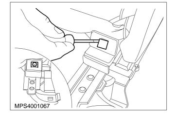
3. Remove the two bolts and tilt back the seat assembly.
