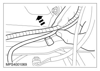
6. Unclip the wiring looms.
