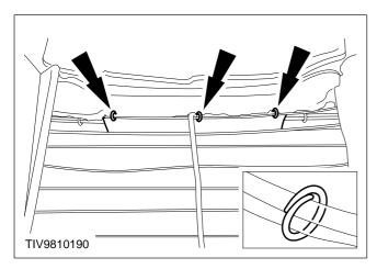
32. Install the three hog rings attaching the rear of the seat cover to the upper edge of the spring frame assembly.
