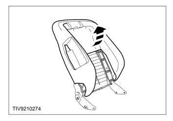
21. Remove the foam pad from the backrest frame.
