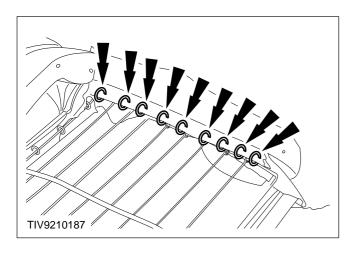
7. Cut the nine hog rings attaching the left-hand side of the seat cover to the spring frame assembly.
