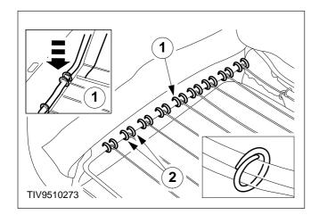
CAUTION: DO NOT reduce the number of hog rings if the seat is equipped with a lumbar mat, 18 hog rings must still be used.
