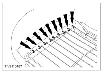
8. Cut the nine hog rings attaching the right-hand side of the seat cover to the spring frame assembly.
