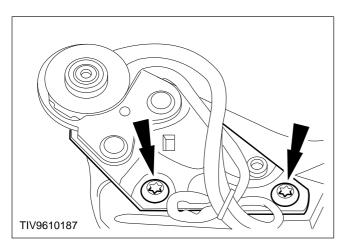
CAUTION: Note the routing of the air bag wiring harness, and power seat wiring harness (if equipped).
