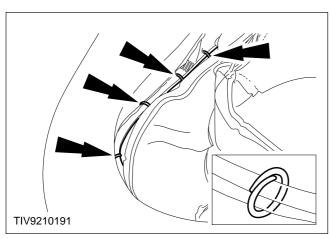
24. Install the four hog rings retaining the left-hand edge of the seat cover to the seat frame.
