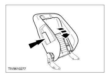
CAUTION: Make sure the opening for the side air bag is correctly fitted around the air bag module.
