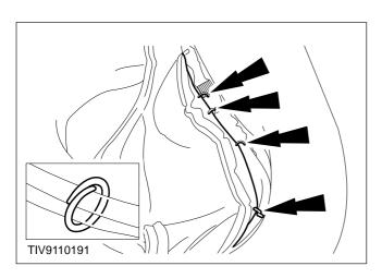
25. Install the four hog rings retaining the right-hand edge of the seat cover to the seat frame.
