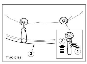
**NOTE:** Rolling the seat cover off the top of the seat frame allows unrestricted access to the hog rings.
