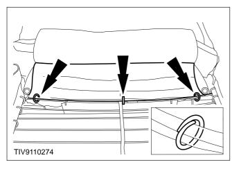
34. Install the three hog rings attaching the heater mat to the upper edge of the spring frame assembly.
