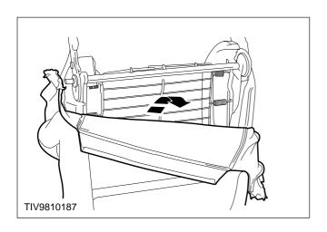
**NOTE:** Rolling the cover off at this stage allows the cover to be inverted allowing unrestricted access to the top of the seat frame later.
