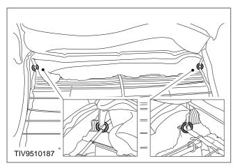
13. Remove the hog ring from the left and right-hand side of the top edge of the spring frame assembly.
