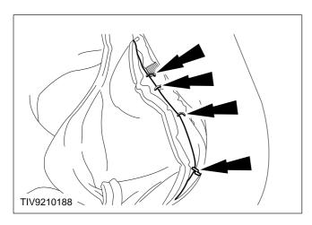
17. Remove the four hog rings retaining the left-hand edge of the seat cover to the seat frame.
