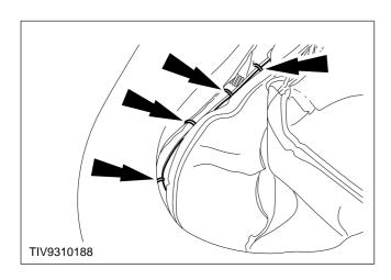
18. Remove the four hog rings retaining the right-hand edge of the seat cover to the seat frame.
