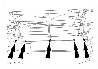
15. Remove the five hog rings attaching the seat cover to the upper edge of the seat frame.
