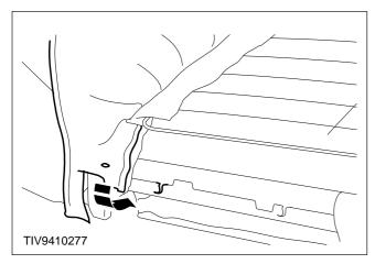
6. Detach the fabric flap on the base of the left and right-hand side of the backrest cushion.
