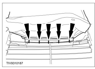
10. Cut the five hog rings attaching the front of the seat cover to the upper edge of the spring frame assembly.
