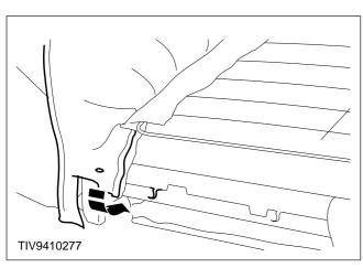
CAUTION: Carefully pull the cover into position over the cushion, making sure the cover seams align with the contour of the seat foam.
