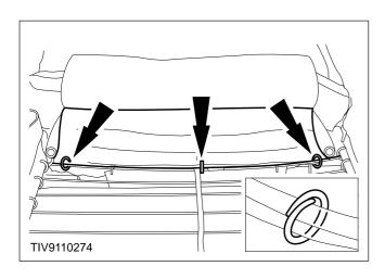
Cut the three hog rings retaining the heater mat to the upper spring frame assembly.
