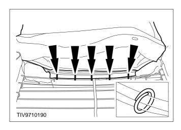
33. Install the five hog rings attaching the front of the seat cover to the upper edge of the spring frame assembly.
