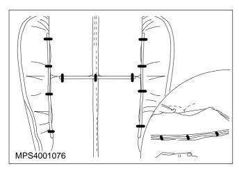
8. Remove the seat cover from the foam backing (11 hog rings).
