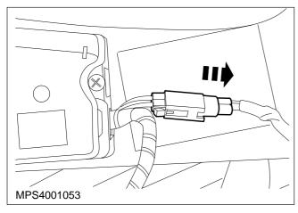
3. Disconnect the multiplug and remove the seat side trim.
