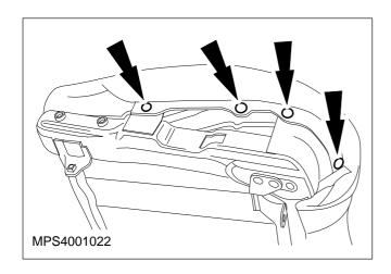
5. Remove the four stud fasteners.
