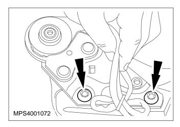
4. Separate the seat cushion and seat back (two Torx bolts on each side).
