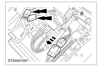
9. Disconnect the main power loom and unclip the two connectors.
