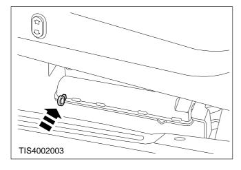
4. Remove the rear side bolt cover (one screw).
