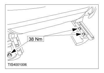
6. Remove the front securing bolts.
