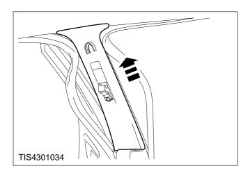
5. Remove the trim by gently pulling upwards to disengage the clip.
