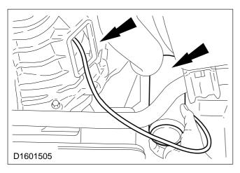
**NOTE:** After bleeding, depress the clutch pedal ten times and check the operation of the system.
