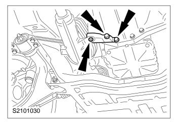
42. Attach the front part of the exhaust system loosely.
