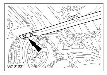
7. Detach the front axle transverse brace (left-hand side shown).
