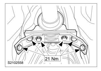
38. Align the centre bearing free of stress and secure it.
