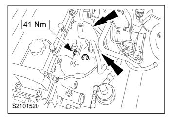
43. Secure the catalytic converter to the exhaust manifold.
