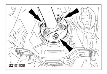
CAUTION: Do not disconnect the driveshaft from the rubber coupling.
