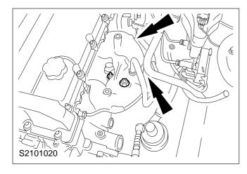
6. Detach the catalytic converter from the exhaust manifold (four nuts).
