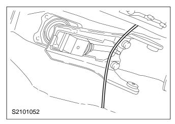
20. Hold the gearshift support bracket in position and support it with a length of round steel rod.
