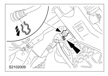
**WARNING:** Seal the line ends with suitable plugs.
