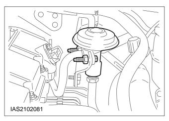
44. Locate the exhaust gas recirculation valve (EGR valve) in position and attach it to the engine.
