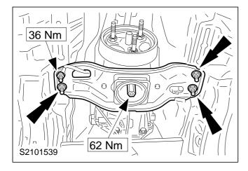
34. Attach the transmission crossmember to the transmission and floor assembly.
