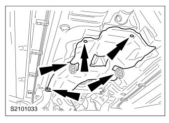
39. Fit the exhaust system heat shield.
