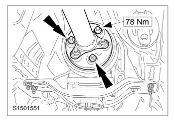
36. Attach the driveshaft to the vibration damper.
