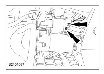
41. Connect the starter motor wiring.
