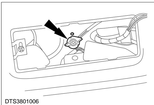
**NOTE:** The antenna mast unscrews from the antenna base.
