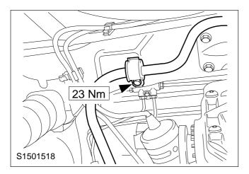
9. Attach the left-hand stabiliser bar mounting bracket.
