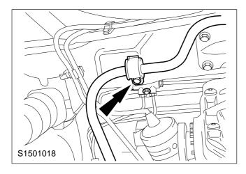
3. Detach the left-hand stabiliser bar mounting bracket.
