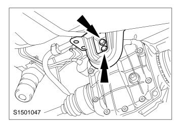
5. Detach the mounting from the cover of the differential assembly.
