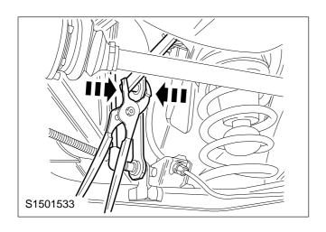
**NOTE:** Connect the ball coupling to the linkage when self-levelling suspension is fitted.
