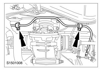
3. Unscrew the stabiliser bar from the floor assembly (two mounting brackets) and remove it (vehicle shown built up to Dec '95).
