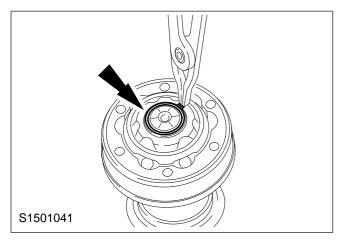
2. Detach the constant-velocity joints from the rear axle driveshaft.
