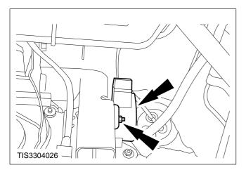
3. Remove the sensor (two nuts).
